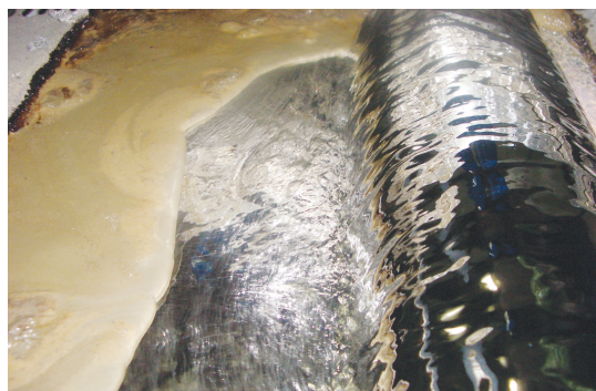
Lead-free solder bath with MS2® molten solder surfactant, showing no dross—only shiny solder
