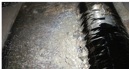
Lead-free solder bath without MS2® molten solder surfactant, showing typical dross buildup
